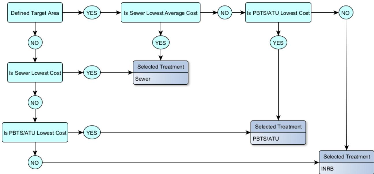
Figure 3. Flow chart with queries to identify recommended AWTS based on cost-effectiveness.
