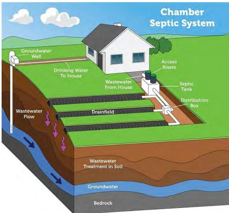
Please note: The ends of the chamber system lines are open for illustrative purposes only. In reality, and when properly installed, these lines are closed at the end. Septic systems vary. Diagram is not to scale.
